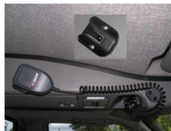
Install microphone clip on acute angle
