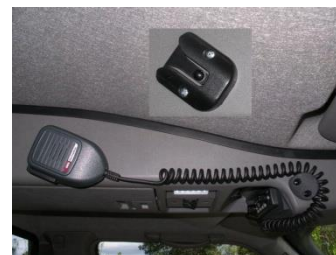
Install microphone clip on acute angle
