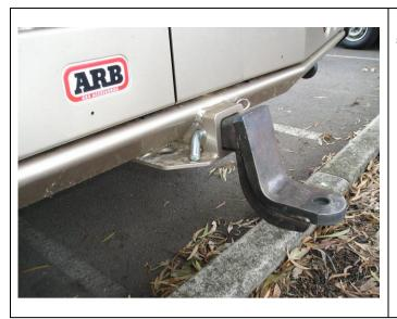
59. Fit gooseneck with pull pin and spring clip as shown.
