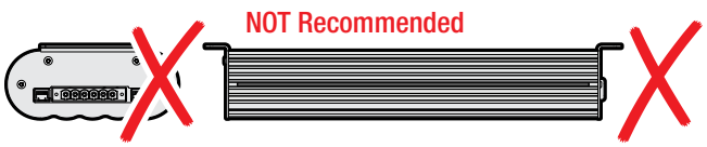
FIGURE 2.2.1.3: Do NOT mount the unit upside down
