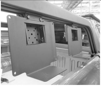
Fit Case mounting plate over mounted brackets as shown using four M8 Flange head bolts. Leave loose.
