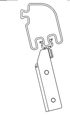
3. Install mount to internal dovetail.
