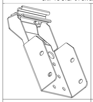
4. Assemble 3752562 to 3755837 as shown using two coach head bolts, M8 nyloc nuts and thin washers.
