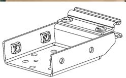
Assemble 3752562 to 4655414 as shown using two coach head bolts, M8 nyloc nuts and thin M8 washers. Ensure the head of the bolts are in the location shown.
