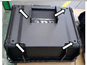
1. Using the 6582535 mounting bracket as a template, drill Ø8.5mm holes in each corner. Remove brackets and deburr all holes.
