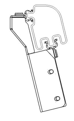
5. Fit larger mount over mount fitted in step 3, tighten M8 nyloc nuts to hold assembly in place.
