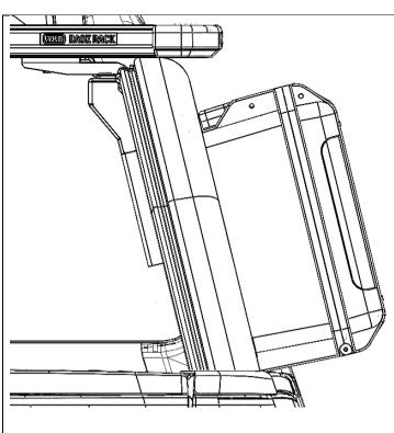
14. Align the case to be parallel with the Bed Rack frame and torque the four M8 flange headed bolts to spec.
